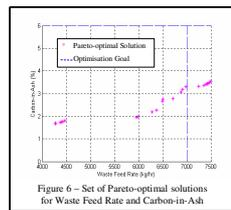
Figure 6 – Set of Pareto-optimal solutions for Waste Feed Rate and Carbon-in-Ash
