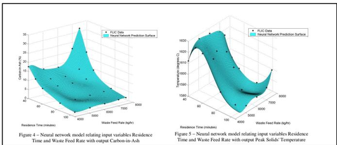
Figure 4 – Neural network model relating input variables Residence Time and Waste Feed Rate with output Carbon-in-Ash
