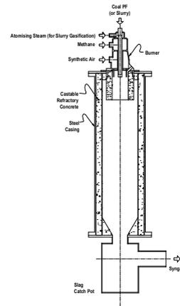
Figure 5: Cross-Section of the USS Gasifier
