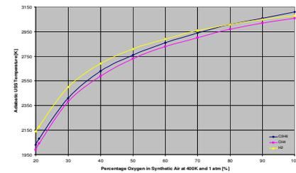
Figure 3: Adiabatic USS Temperature vs Synthetic Air Composition
